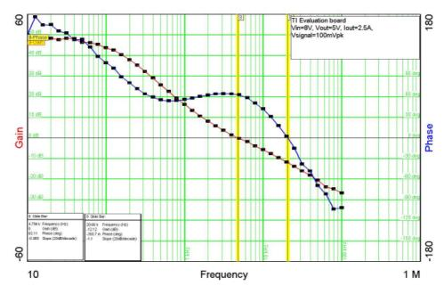
Venable plot at Low-line at load of 2.5 A, Vsignal = 100 mVpK. The Venable injection transformer has a 10 to 1 turns ratio so the real injection voltage is 10 mV peak. Crossover or bandwidth is 4.79 KHz with a PM of 63.1 deg while GM = -12.12 dB
