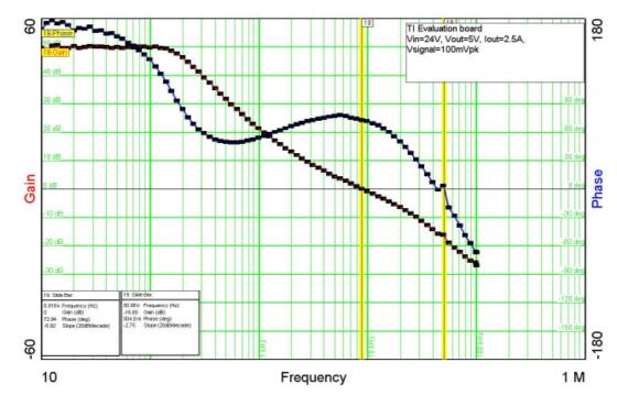
Venable plot at High-line at load of 2.5 A, Vsignal = 100 mVpK. The Venable injection transformer has a 10 to 1 turns ratio so the real injection voltage is 10 mV peak. 0 dB gain at 8.9 kHz (phase = 72.8 deg), 0 deg phase at 50.9 kHz (-16.6 dB gain).
