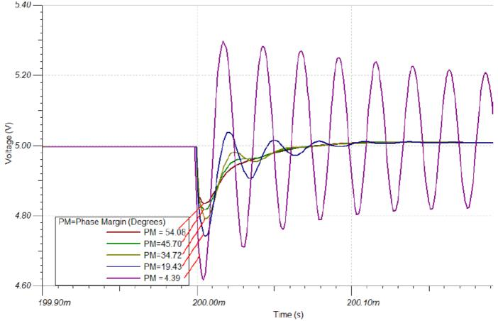
Here is a plot of output voltage in response to a Load Step with different phase margins:
