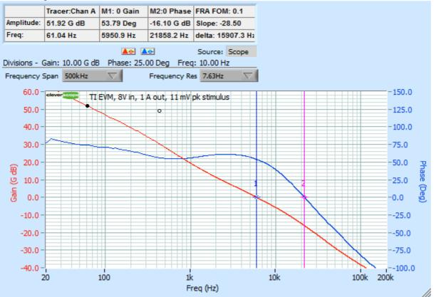
0 dB gain at 5.9 kHz (54 deg) and 0 deg phase at 21.8 kHz (gain is -16.1 dB).
