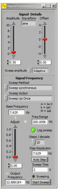
The Signal Generator is set to sweep the signal range with a log sweep. It uses 20 steps per decade.
