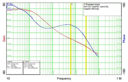
We see 0db gain at 6.2kHz (69 deg phase margin) and 0 deg phase at 30 kHz (-13 dB gain margin). These are similar results to both the Cleverscope and TI network analyser results. (If anything the Cleverscope results are closer).
