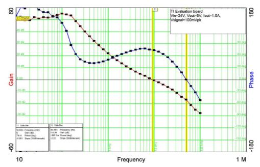
Venable plot at High-line at load of 1.0 A, Vsignal = 100 mVpK. The Venable injection transformer has a 10 to 1 turns ratio so the real injection voltage is 10 mV peak. Crossover or bandwidth is 9.45 KHz with a PM of 74.4 deg while GM = -16.94 dB
