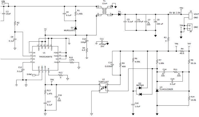
Here is the circuit diagram for a typical isolated flyback converter, this one using the TI TPS55340:
