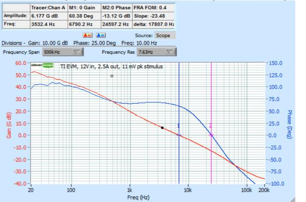
The Cleverscope 0dB gain is 6.8 kHz (60 deg phase phase) and 25.6 kHz phase (-13.1 dB gain margin). These results, and the shape of the graph are very close to that of the TI network analyser.
