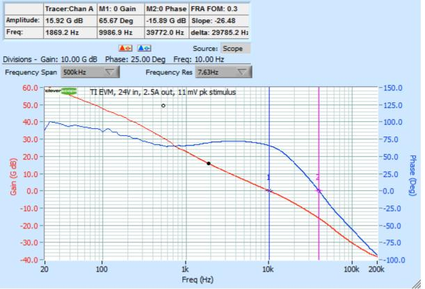
0 dB gain at 10 kHz (66 deg) and 0 deg phase at 39.7 kHz (gain is -15.9 dB).
