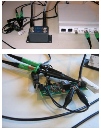
The test signal was injected across R3, using TP2 and TP6. R3 was changed to be 50 ohms. The CS328A signal generator, isolated using the VB-1BB transformer fed via a 20 dB attenuator (x 0.1) supplied the test signal. The test signal amplitude was about 13 mV peak. The signal was swept from 20 Hz to 200 kHz. The VB-1BB showed no sign of saturation until below 20 Hz. Injecting across R3 allows the regulator feedback loops to be stimulated.
