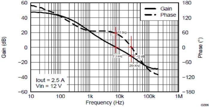
Here we estimate 0 dB gain at 7.2 kHz (59 deg phase) and 0 deg phase at 25 kHz (-12 dB gain).
