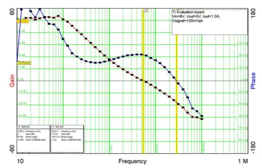
Venable plot at Low-line at load of 1.0 A, Vsignal = 100 mVpK. The Venable injection transformer has a 10 to 1 turns ratio so the real injection voltage is 10 mV pk. Crossover or bandwidth is 5.48 KHz with a PM of 64.3 deg while GM = -17.87 dB
