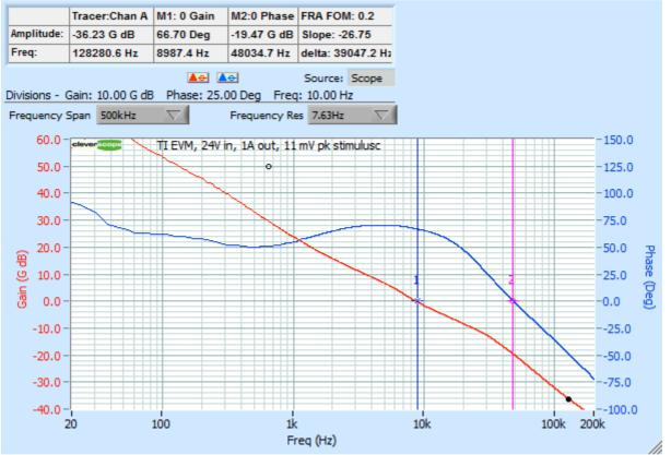
0 dB gain at 8.9 kHz (67 deg) and 0 deg phase at 48 kHz (gain is -19 dB).
